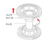
Slide the film into the reel with the emulsion side facing the centre. Start with the inner-most slot.
