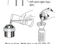
Pour in fixer. Refit the push-on cap 1 and invert once every 60 seconds. After the full fixing time remove the cover 1 and pour out the fixer.
